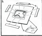
Below—right: How to make a light box top. A. Cut hole the size of glass in middle of board. B. Nail wood strips (to hold glass) beneath holes. C. Put in glass (which should be as thick as the board).
